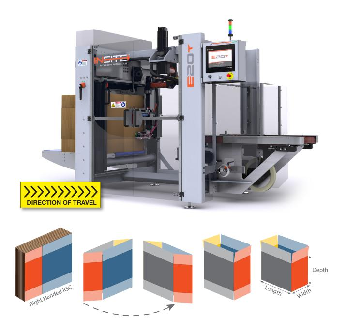
When looking at the HMI, *Right Hand* machines move *Right Hand* cases from left-to-right as they are erected and sealed.
