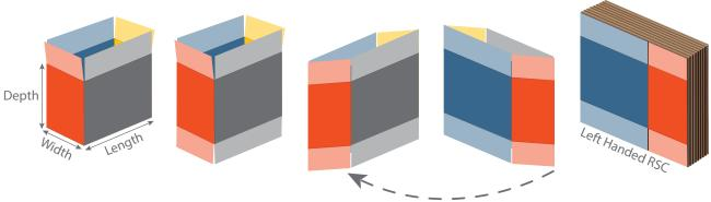
When looking at the HMI, *Left Hand* machines move *Left Hand* cases from right-to-left as they are erected and sealed.
